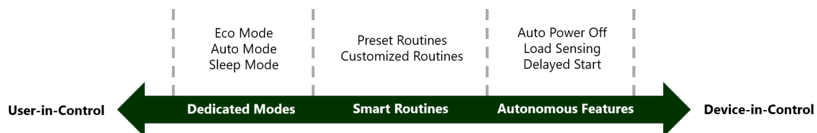
Fig. 1. Common home appliance ESFs categorized according to the level of user control they provide. ESFs that provide the most user control are dedicated modes integrated into the device. Contrary, autonomous functions are commonly entirely controlled by the appliance. Smart functions provide the ability to select predefined smart routines or create customized routines.
