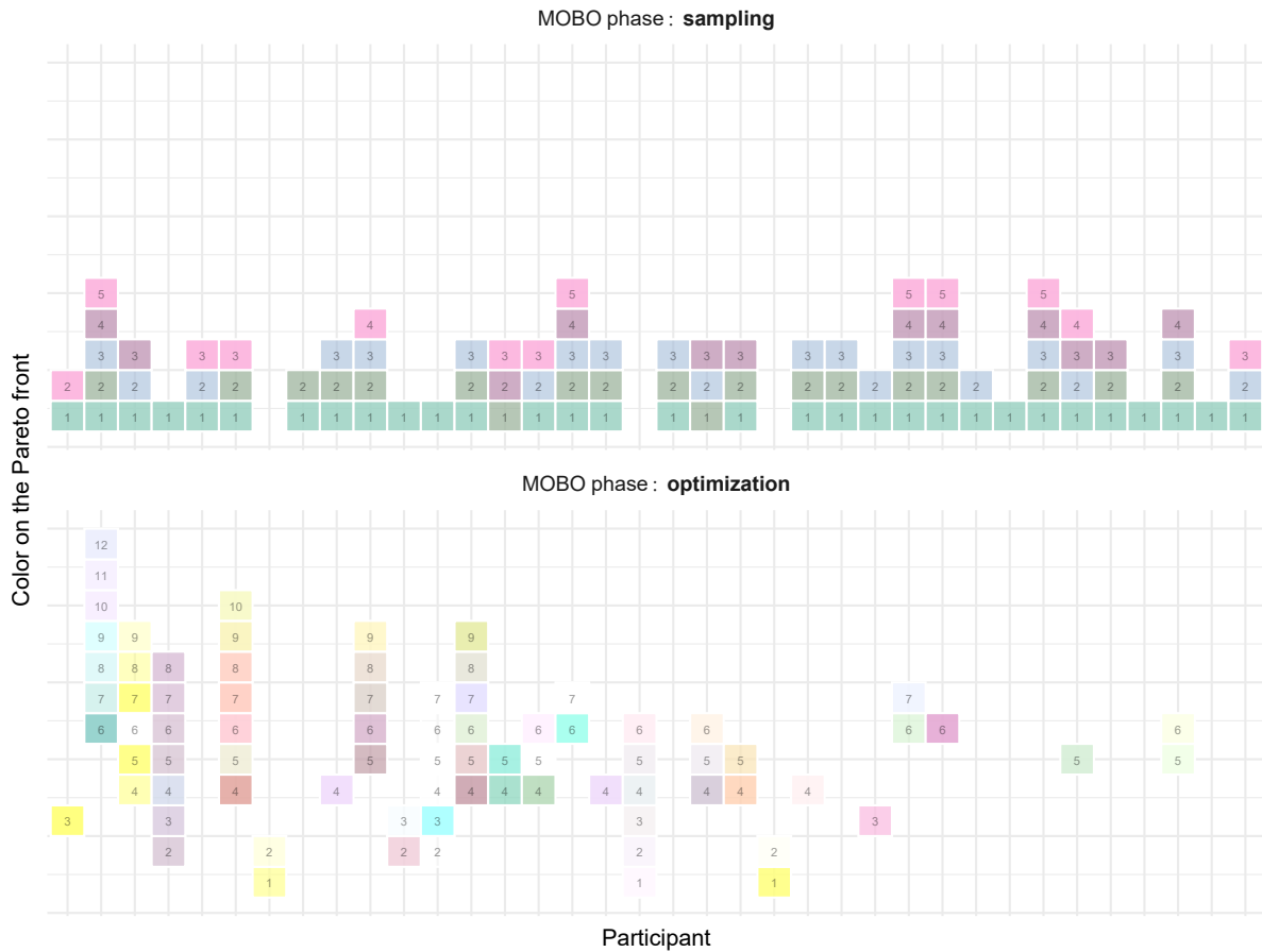
Figure 9: Color distribution for the Pareto front, split into sampling (1-5) and optimization (1-15) phases. The number in a box indicates the iteration in which this color was set, counting from the bottom. The columns on the x-axis represent the individual participants. An empty spot in a column means this iteration was not Pareto-true (i.e., dominated by another design).
