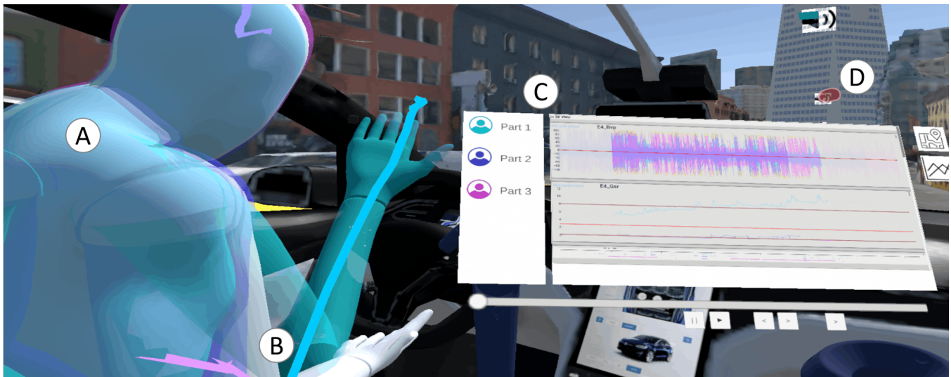
Figure 3: The AUTOVIS VR view provides an interactive study replication. A virtual tablet showing physiological data is attached to the left VR controller with a timeline for scene playback. The VR view hosts a virtual replication of the ego vehicle, passenger movements as avatars and trajectories, and gaze, touch, and pointing as heatmaps in the interior and environment.
